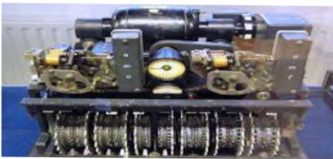
German Lorenz cipher machine, used in world war II to encrypt very-high-level general staff messages
