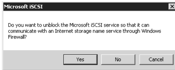
FIGURE 10-13 Unblocking the iSCSI Service on the client computer
